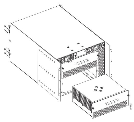
Figure 39. Blower assembly removal and replacement
